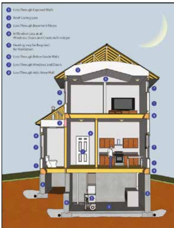
Figure 5. Heat Loss Locations
